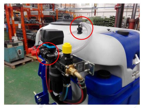
5. Then, connect the two small hoses as the picture. Important! <u>The hose with the red</u> <u>mark must go to the right way!</u> The hose with the elbow connection goes as the picture.
