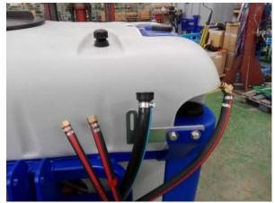
3. Now fix the electro valves kit with the screws of the filter holder in the same position as the picture.
